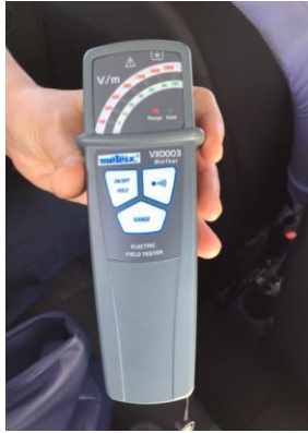
Fig. 1 BIOTEST VX0003 electric field measuring device
